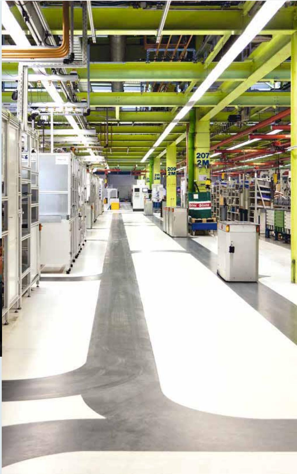
MOVITRANS® is made up of stationary and mobile components for contactless power supply to moving electrical loads. The required energy is transferred via electromagnetic fields (contactless) from a coil or an insulated stationary conductor via an air gap to the mobile consumers (vehicles) either selectively at specific points or along a track. Compared to conventional energy transfer, e.g. using contact lines or charging
